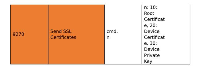
So, for sending the Root Certificate we should enter the command 9270,10 in the terminal.
