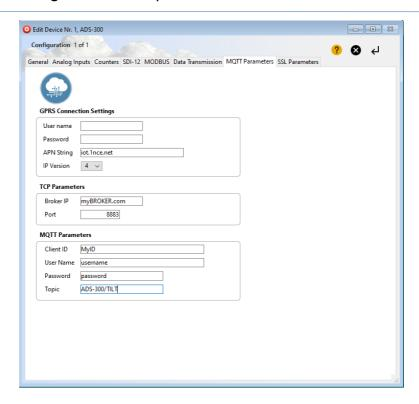
Lastly, in the SSL Parameters tab, we copy and paste the three files needed for the TLS communication: Server Certificate (CA), Device Certificate and Device Private Key.
